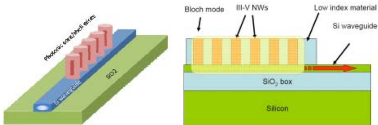
Figure 7: Schematic view of a resonant light source based on 1D array of photonic core-shell NWs on top of a SOI waveguide.
